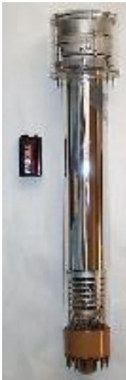
The camera tube measures 390x75mm overall (50mm across the main body)
