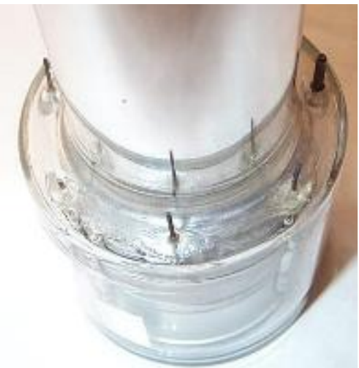
The tube has a 14-pin base and 7 connections around the image section at the front.
