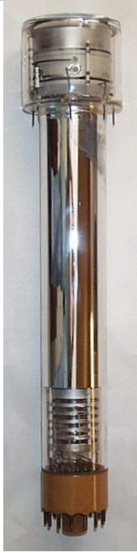
The camera tube measures 390x75mm overall (50mm across the main body)
