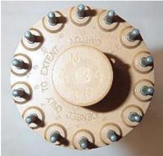
The tube has a 14-pin base and 7 connections around the image section at the front.
