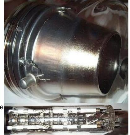
At the other end is a normal looking electron gun. The tube deflection is electromagnetic.
