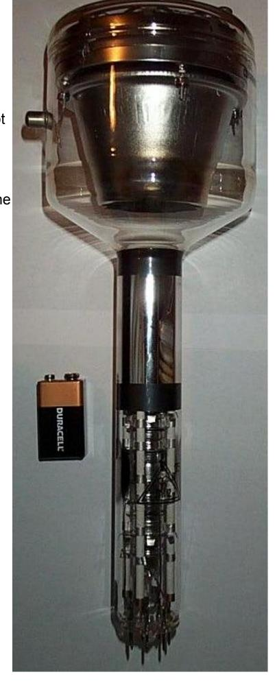
The middle connector connects to the disk (where the screen should be!) and the outer connector connects to a metal ring.
