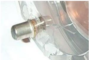
This cone is behind the disk and connects to a connector on the side of the tube. There are no other connections to the cone.
