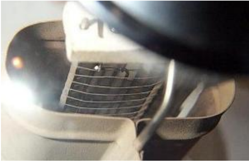
A view down into the valve showing the grid and the thick filament wires, and (below) the grid and filament connections.
