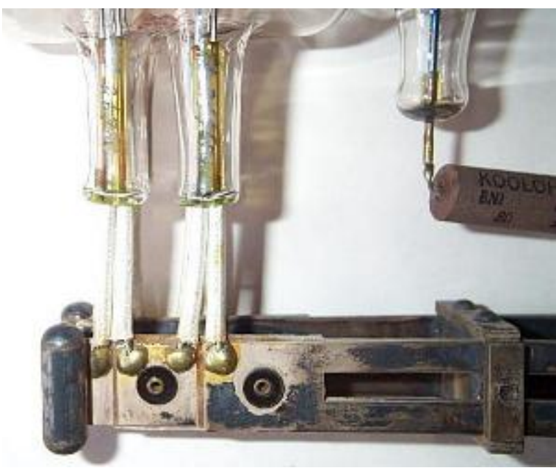
Above and below: the 600MHz tuneable resonant line.
