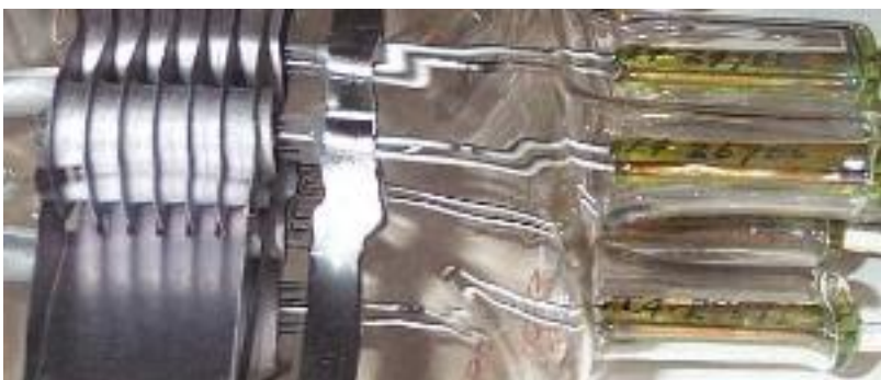
Above: the filament lead seals are all individually labelled. The markings are: I4-24968, I4-26786, I4-27641 and I4-27642.
