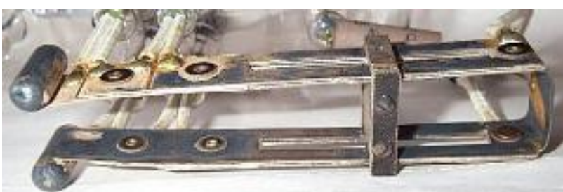
Above and below: the 600MHz tuneable resonant line.
