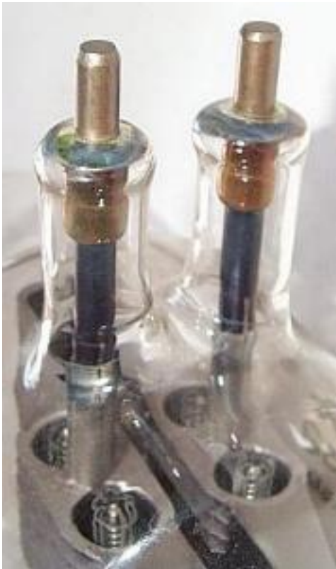
Below: closeup of the balanced anode lines.
