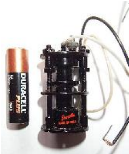
This valve measures 56x30mm overall
